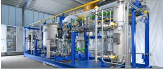
Pre-manufacturing of skid in CALORIC's production facility
