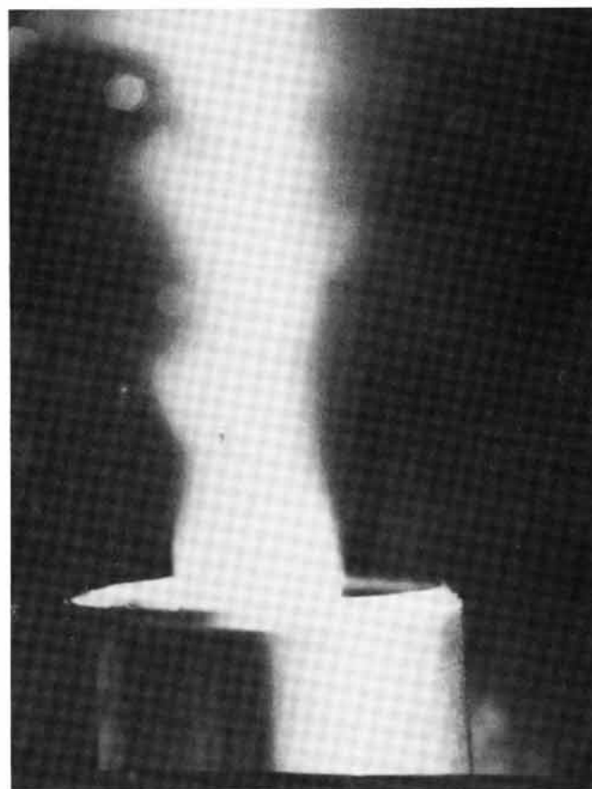
Fig. 4: Atomization of liquid waste by means of high frequency oscillation.
