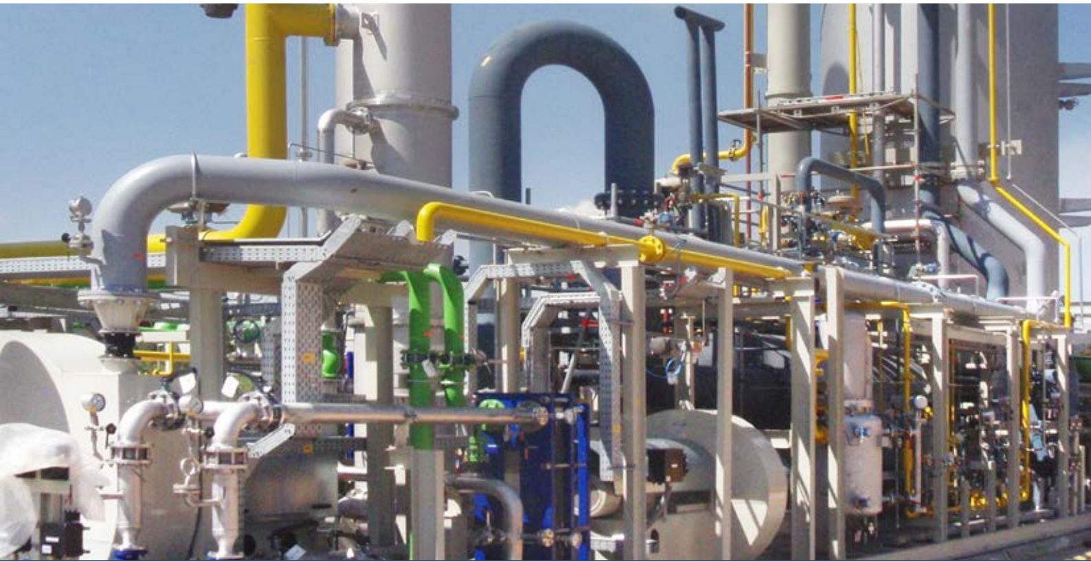
Calcor® plant for 530 Nm 3 /h
