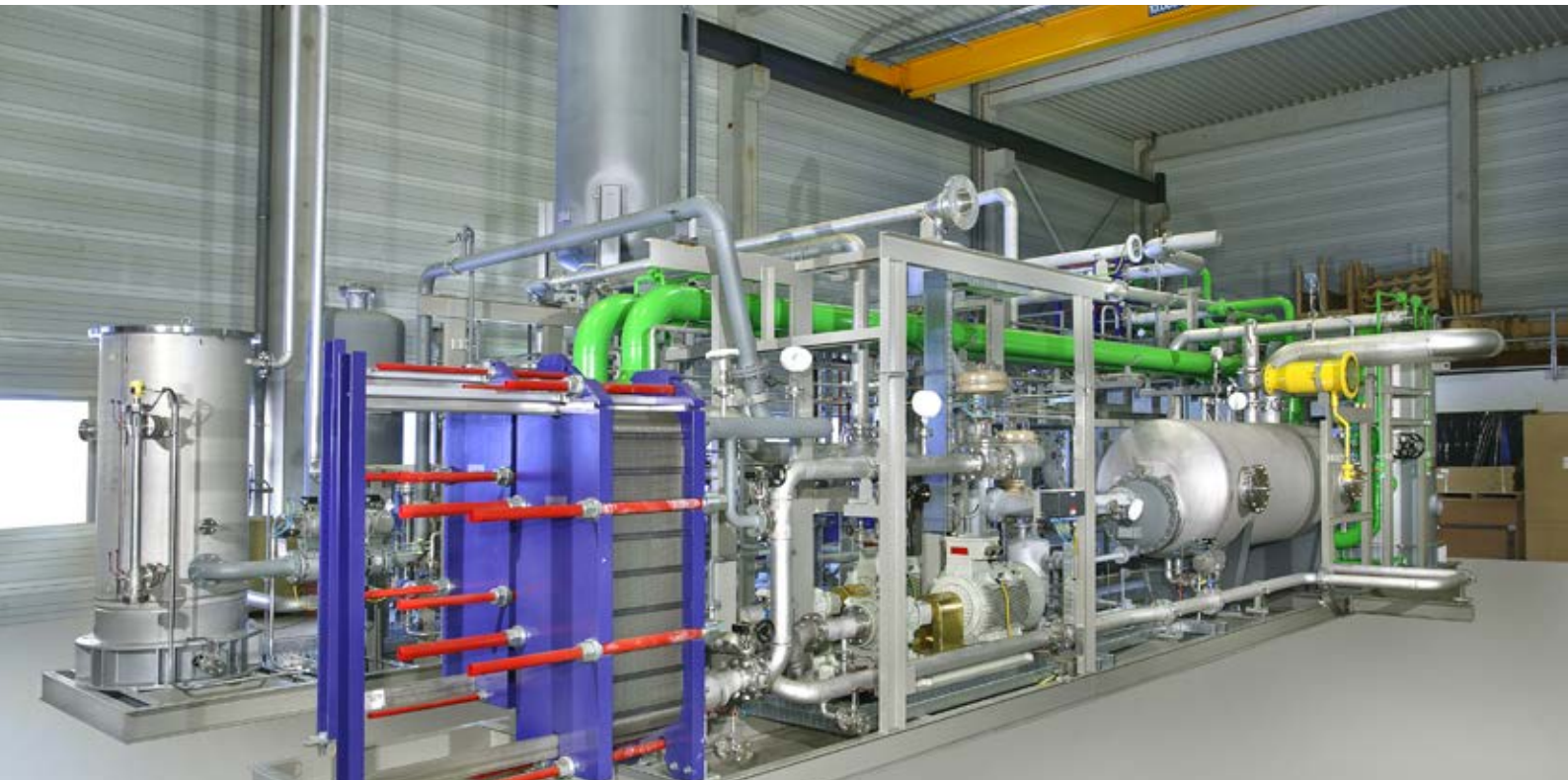
Amine recovery skid during manufacturing
