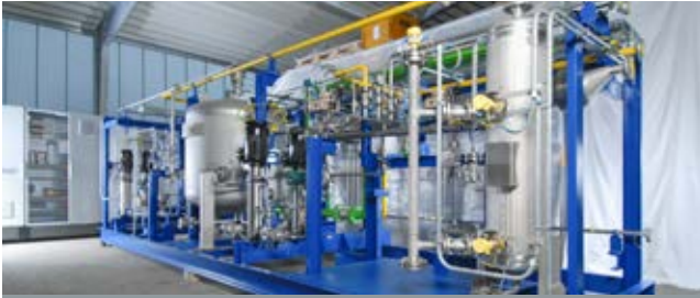
Pre-manufacturing of skid in CALORIC's production facility
